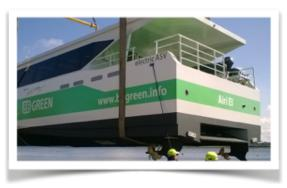
The prototype, which was built in Riga, has dimensions of  $20 \times 6$  m, a capacity of 80 passengers and needs a power of 600 kW (Propeller + fan) to make 30 knots. During the development, 2000 tank tests were carried out with different models at SSPA in Gothenburg before the best dimensions could be determined. The extensive material and comparisons between theory and full-scale prototype makes it possible to scale-up the ship to larger dimensions with a tolerance of +/-5%.
