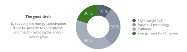
The total energy savings are 80%. In hydrogen operation, the efficiency is less than for batteries - 50%, which means energy savings of 65%.
